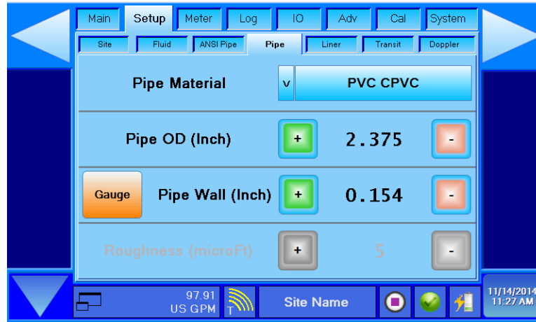
Figure 55: Pipe page allowing manual entry
