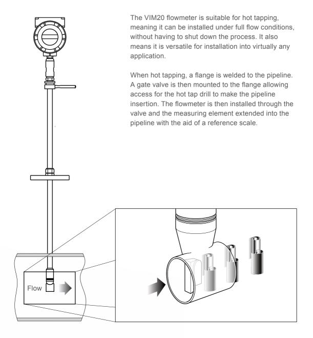
As the VIM20 can be fitted directly into operational pipework, installation is quick and easy without process shutdown. The cost of labour is reduced and data can be gathered more swiftly. Typical savings can be as much as 80% for DN600 pipelines and 50% for the DN250 pipelines.
